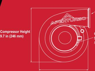
**Compressor Outlet** 4.21 in (107 mm) v-band attachment
